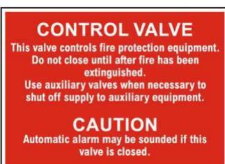
NFPA 13 Section 7.7.1.5.2 The caution sign shall be worded as follows: This valve controls fire protection equipment. Do not close until after fire has been extinguished. Use auxiliary valves when necessary to shut off supply to auxiliary equipment.
