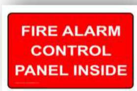
Rooms containing the "Fire Alarm Control Panel" shall be provided signage a minimum of 7” high by 10” width with 2-inch high block letters a 0.5” letter stroke - white letters on a contrasting red background. and shall be permanently attached, at normal eye level to the door leading to the fire alarm control panel(s) unless otherwise approved by the Office of the Fire Marshal.
